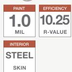
2" thick insulated steel sandwich panel constructed of top quality materials. Flush panel with deep woodgrain texture and two coat prefinished paint system all combine to enhance the beauty of your home.
